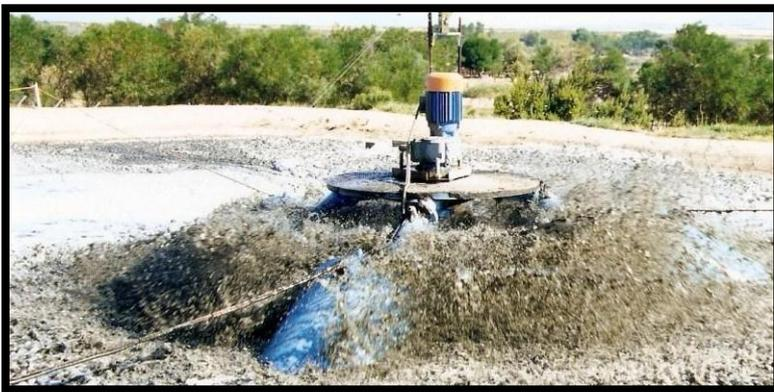
Surface aeration is an economical method to aerate a large body of water such as a dam or pond. For a bioreactor using surface aeration, the geometry of the bioreactor is extremely important. To achieve good oxygen transfer the bioreactor needs to be cylindrical in shape with a slightly coned shaped base.
